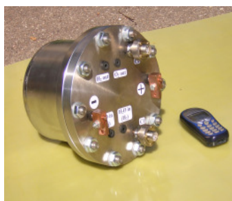
Fig. 1. Fuel cell with power up to 5 kW and electrolysis battery productivity up to 1 m 3 /h (working pressure 3 MPa). Research was is executed at financial support of FASI (Rosnauka)
