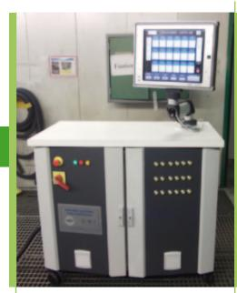
MAXIM induction heating power supply and control unit with associated "butterfly" type coil, developed within the frame of the INDUCTOR project for heating of composite repairs
