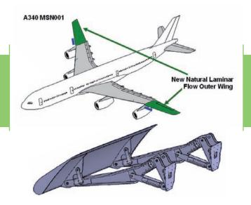
Example of one of the two Krueger flaps (below), designed and manufactured by ASCO Industries for flight testing on a modified A340-600 by Airbus (above).
