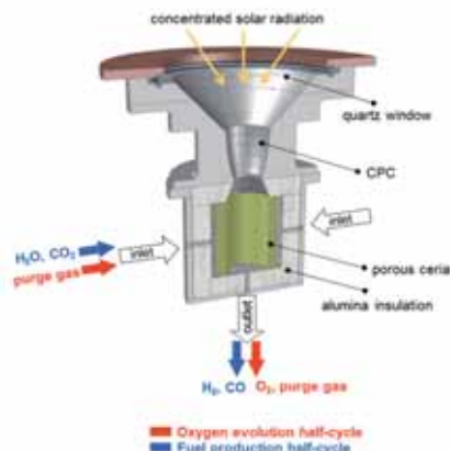
Schematic of solar reactor for the two-step thermochemical production of syngas (carbon monoxide and hydrogen, a precursor for solar jet fuel) from carbon dioxide, water and concentrated sunlight (Chueh, W. C., Science 2010, 330 (6012), 1797-1801.)
