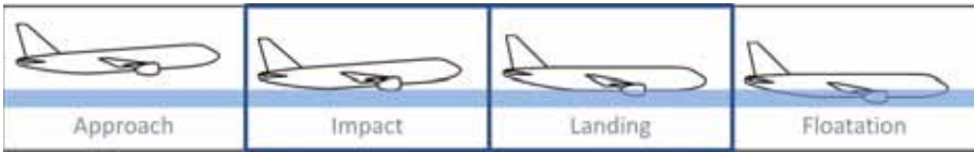
Phases of aircraft ditching
