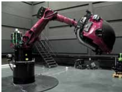
MPS cyber motion simulator that is used for scientific research in motion perception, flight training, simulating aviation and driving experiences
