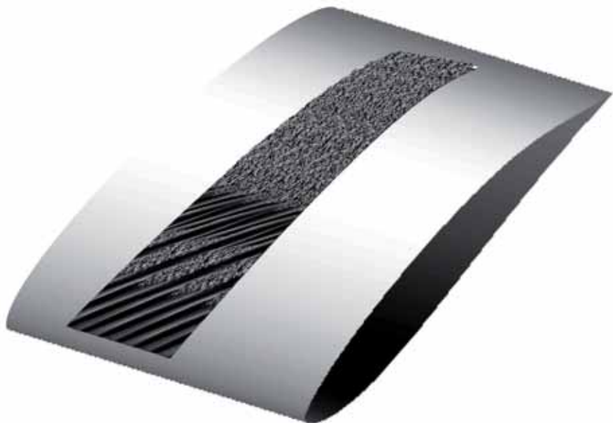
Direct numerical simulation of cross-flow transition on a swept wing
