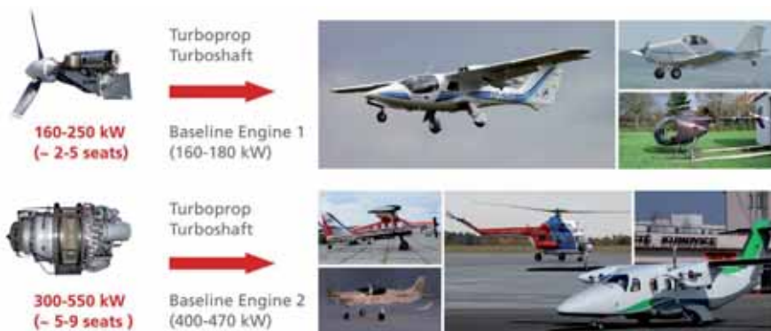
Categories of propulsion units and their possible application
