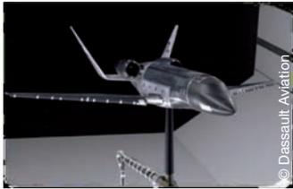
The empennage shields the engine noise from the ground.
