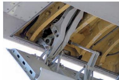
**Classical slat system with actuation system visible:**
