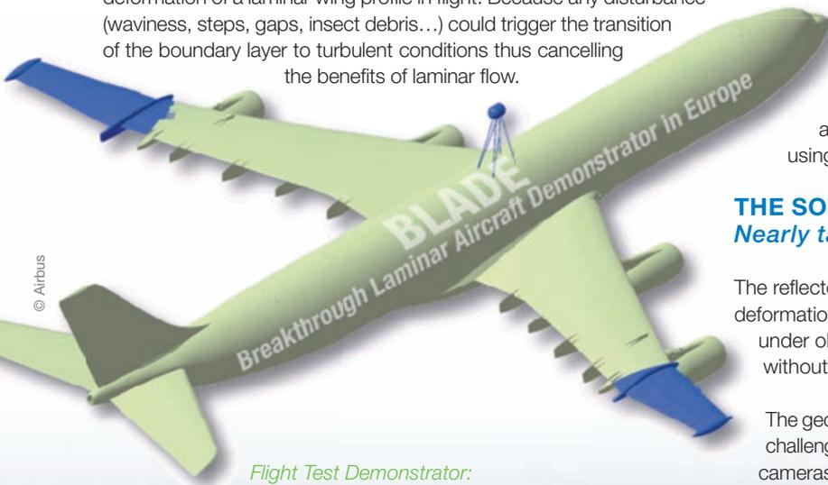
*Flight Test Demonstrator: an A340-300 has been selected as platform; the outer wing (blue areas in the picture) will be replaced with the new laminar wing sections.*
