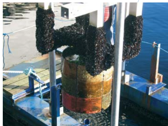
Performance test of marine antifouling paint systems
