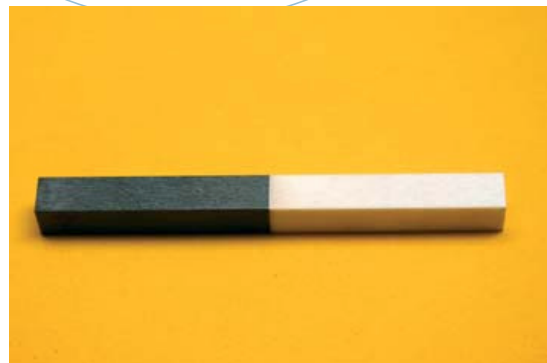
2C-CIM testing component consisting of black and white zirconia
