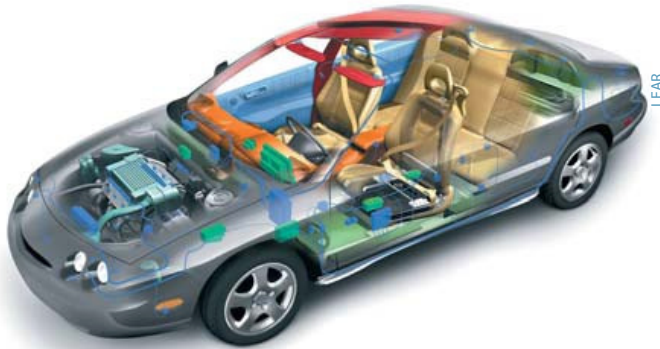
Schematic illustration of the automotive electrical and electronic system (EES)
