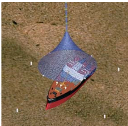
DIFIS system dome covering a wreck at the sea bottom
