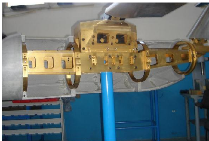
Figure 2: model suspension system (vertical strut)
