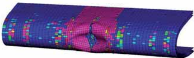
Simulated impact damage of a sandwich structure.
