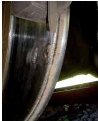
Typical flat defect on wheel
