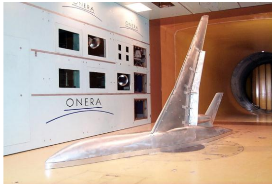
Figure 1: Provided generic Falcon fuselage with nacelles with a generic Falcon Wing
