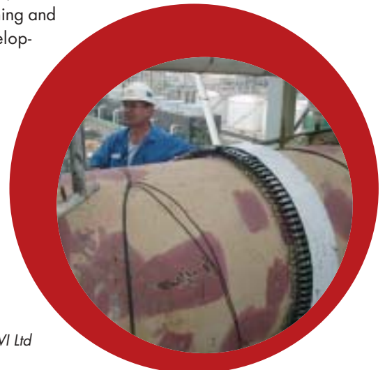
Teletest tool mounted on a 1.2m-diameter pipe in a refinery, to examine for corrosion.
