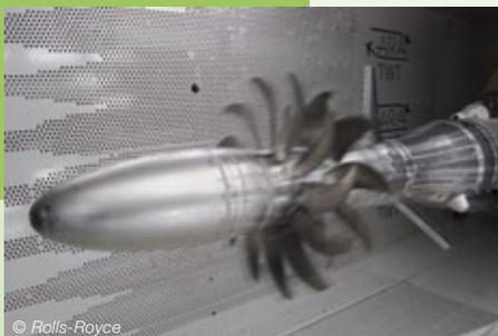
Rolls-Royce first performed extensive tests of a contra-rotating open rotor (CROR) in the 1980s when they commissioned a new purpose-built rig (rig 140) which was tested at the ARA wind-tunnel in Bedford (UK).
