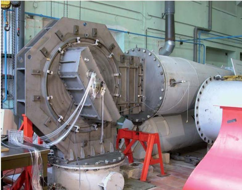
Cascade test section in the wind tunnel at VKI
