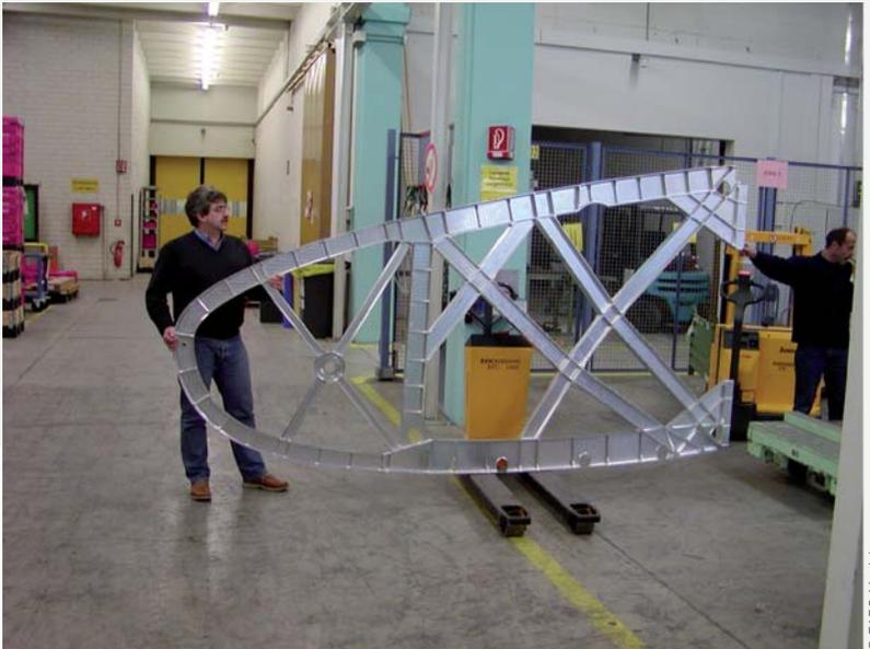
A topology optimisation-based design for integrally stiffened machined ribs for the inboard inner fixed leading edge of the Airbus 380
