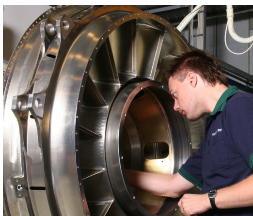
Figure 1. Example of welded Turbine Exhaust Case including forged parts
