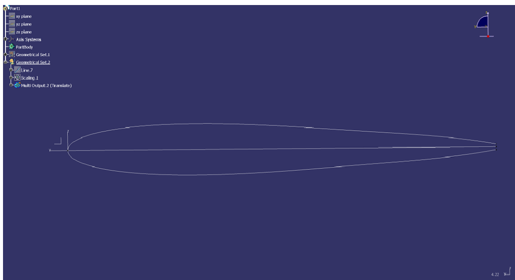
Figure 7 Enlarged trailing edge thickness for the Gurney flap region
