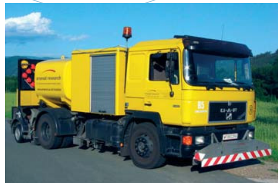
Recording of surface and road parameters
