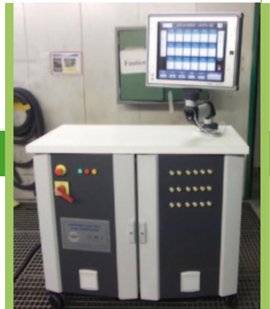
*MAXIM induction heating power supply and control unit with associated "butterfly" type coil, developed within the frame of the INDUCTOR project for heating of composite repairs*
