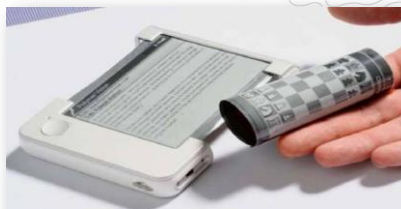
Figure 1: Photograph of Polymer Vision display, in rolled-up state and integrated in product prototype.
